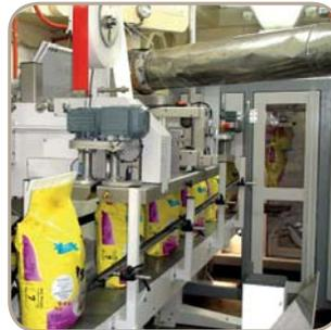
Statec Binder bag closing machine SBSM-OS in operation
