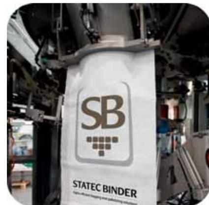
The bagging systems are designed for PE-, woven PP- and paper bags with a filling weight of 5 to 50kg. Big Bag-stations fill up to 150 Big Bags per hour and the palletizing systems are able to stack all types of bags and boxes. With 40 years of experience STATEC BINDER manufactures high-performance open-mouth bagging systems and is known for absolute reliability, innovation and precision.
