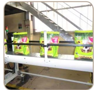
Heat sealed PE bags on belt conveyor
